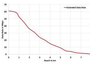
Rate/Reach Performance Measurement of Intel® SHDSL Chipset. Extended Data Rate, crosstalk-cancelled, sequential startup, 4-pair bonding, standard twisted copper pair phone cables, no alien noise
